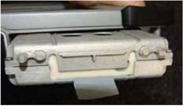
A side view of the hard drive compartment with the drive partially pulled out, showing a white extraction tape.                                    | <p>A continuación, extraiga el disco duro de su compartimento tirando de la cinta de extracción.</p>                                                                                |
