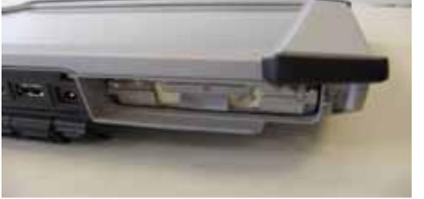
The hard drive is fully inserted into the compartment, and the extraction tape is visible.                                                       | <p>Disco duro completamente introducido y encajado.</p>                                                                                                                             |
