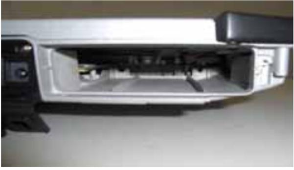
A view of the empty hard drive compartment, showing the internal structure and the extraction tape.                                               | <p>Vista del compartimento del disco duro vacío.</p>                                                                                                                                |
